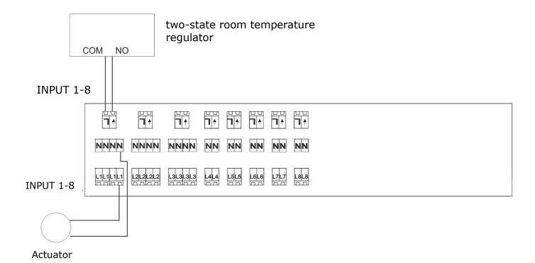
The wiring diagram above illustrates how the room temperature regulators and the actuators should be connected.
